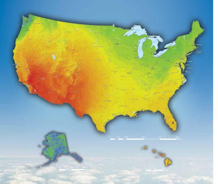
Annual average solar resource data is shown for a tilt = latitude collector. The data for Hawaii and the 48 contiguous states is a 10 km, satellite modeled dataset (SUNY/NREL, 2007) representing data from 1998-2005. The data for Alaska is a 40 km dataset produced by the Climatological Solar Radiation Model (NREL, 2003).
